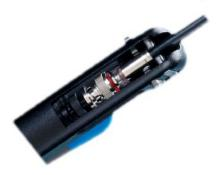
5) Place assembly in compression tool (30-793 shown) and compress.
