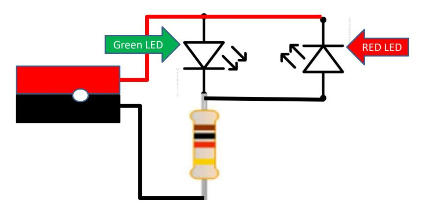
Proper polarity lights green LED Improper polarity lights red LED. Resistor is 1,000-ohm ¼ watt
