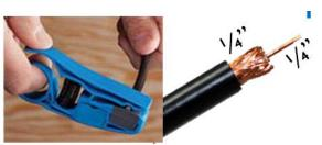
I) Use coax stripper to strip cable so 1/4" of conductor and 1/4" of braiding are exposed. (45-605 shown)
